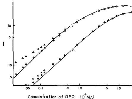
Fig. 1. Comparison of theoretical curves of fluorescence intensity vs. solute concentration with experimental values for the aerated DPO-toluene solutions excited by 260  $m\mu$  UV. Curves A and B are calculated ones, ( $\Delta$ ) and ( $\blacktriangle$ ) are the observed values for  $\text{CCl}_4$  concentration of zero and  $1.7 \times 10^{-3} M/l$ , respectively.
